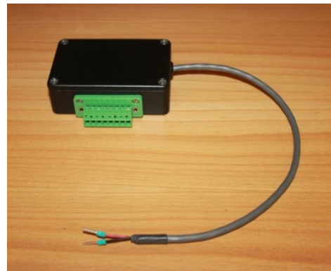
Figure 17: 5VDC expansion box
