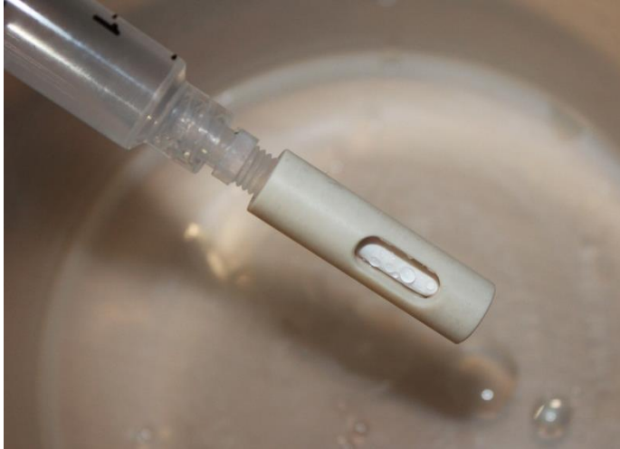
Figure 26: Back flushing a sample probe filter tip
