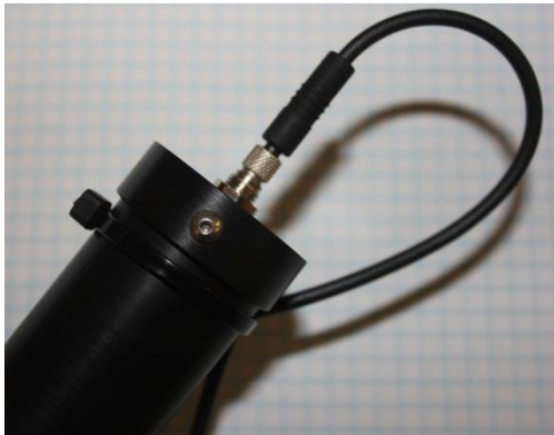
Figure 27: Additional strain relief for the probe cable
